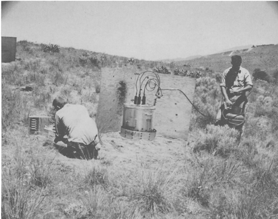
FIG. 3. Propane gas burner with five jets, used to burn plants in situ for 30 sec. One of the five panel meters served to measure magnitude and duration of temperatures.
